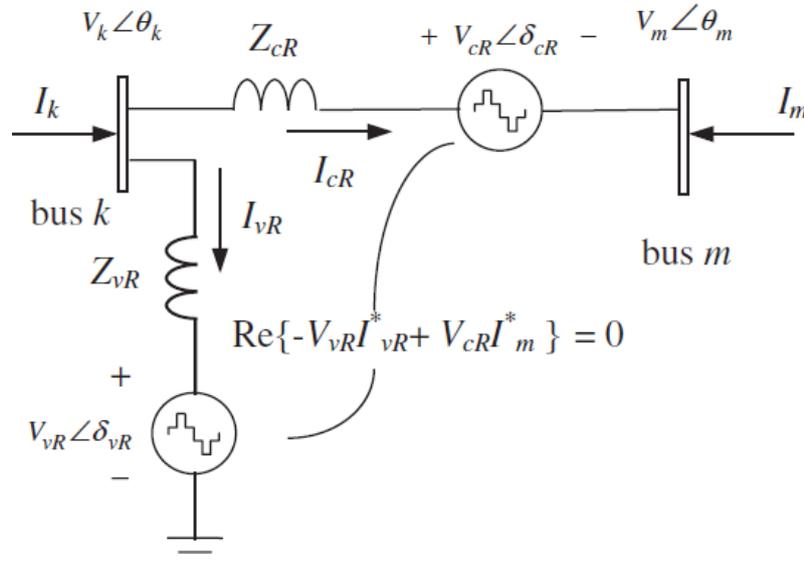
Figure 3: Unified power flow controller equivalent circuit
