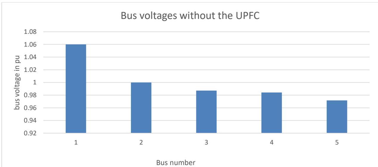
Figure 4: voltages of the buses without the UPFC between buses 3 and 4
