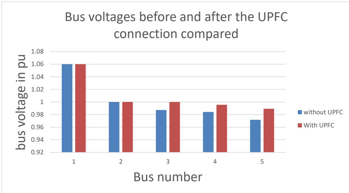
Table 6: voltages of the buses with and without the UPFC between buses 3 and 4
