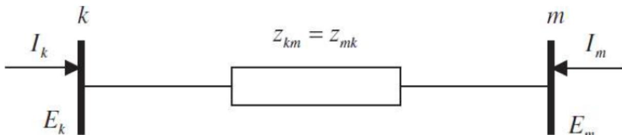
Figure 2: A two bus system for illustrating Newton Raphson Power flows
