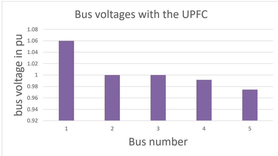
Figure 5: Voltages of the buses with the UPFC between buses 3 and 4
